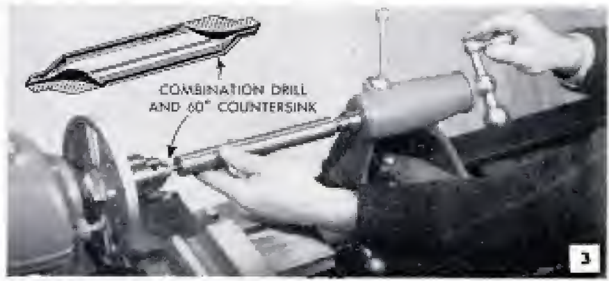
In live drilling, pictured in the photos above and below, the drill usually is held in a geared chuck and driven by the lathe headstock. Flat work is supported by a pad as in the lower views. Note wooden facing
